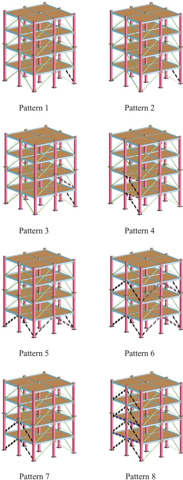
**FIGURE 8** Damage patterns for the SHM benchmark problem
