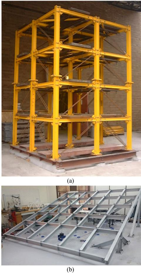
**FIGURE 18** (a) IASC-ASCE SHM benchmark building (photo courtesy Prof. Carlos Ventura, UBC), and (b) QUGS structural steel frame (photo courtesy Prof. Onur Avci, QU)
