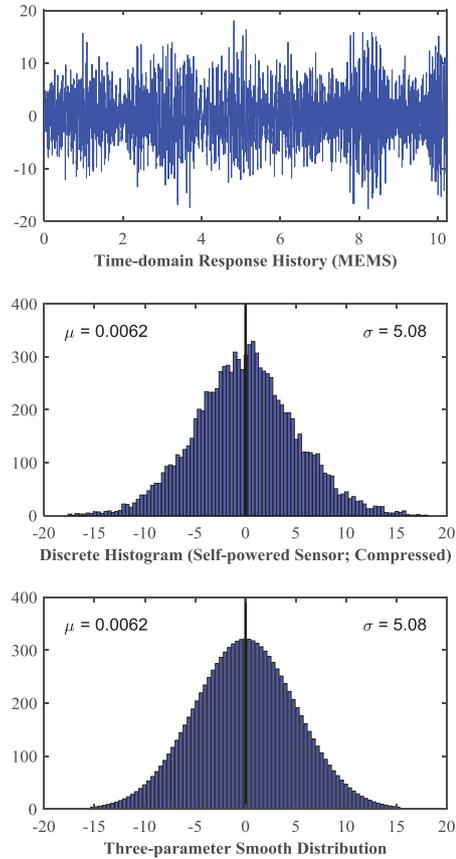
**FIGURE 5** Data compression in the form of histograms (level crossing cumulative time counting) using self-powered sensors
